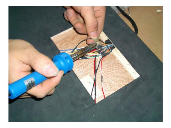
7. Put the insulating tube cover the soldering point, and then hot it up to crimple it.
