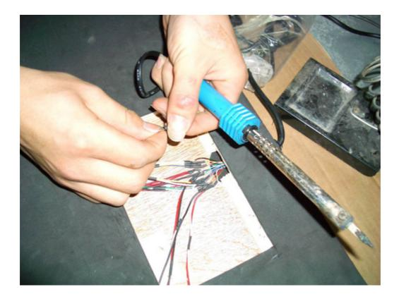
6. Use soldering iron to jointing it well.
